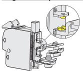
"V-shape" self-cleaning contacts with quadruple contact point. This type of shape, thanks to the presence of the double contact point, makes it possible to drastically reduce the probability of contact commutation failure. In addition to this, it improves considerably the reliability in the presence of dust.
