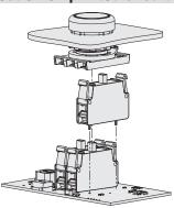
Versions with panel mounting of the EROUND series contact blocks with solder pin are available. If there is no wiring but a printed circuit, these contact blocks can be directly welded on the latter.
