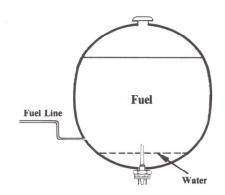
TO DETECT WATER IN FUEL TANKS USE MODEL 613 ( ) H ( )
