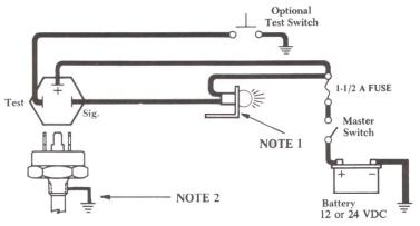
Wiring connections for standard Model  $613/624~N(\ )U$  negative ground vehicles ungrounded loads.
