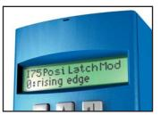
The POSILatch function uses external signals and evaluates them as measurement function.
