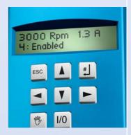
Display and keypad are integrated. So rapid diagnosis, status monitoring, direct parameter access and jogging (manual operation functions) are possible.
