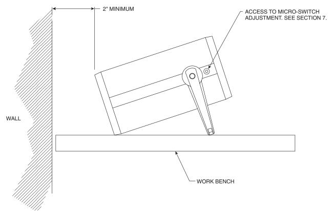
Figure 4. Tilt positioning for operation (side view)
