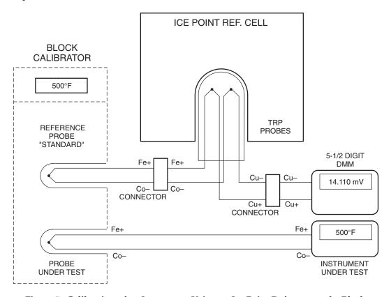
Figure 5. Calibration of an Instrument Using an Ice Point Reference and a Block Calibrator
