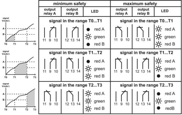
For both output relays, A and B, the safety function can be set separately. This can be carried out by two switches, one per relay, inside the device.
