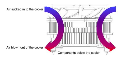
**Note**: The temperature of the air blown out of the cooler should be 70°C maximum.
