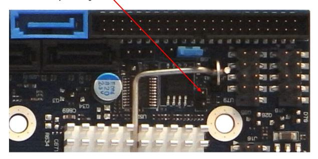
After rebooting, remove the Jumper before Default BIOS is recovered by reloading BIOS (for instance by using latest BIOS upgrade package from web product page).
