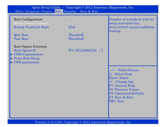
**Note**: When pressing <F7> while booting it is possible manually to select boot device.
