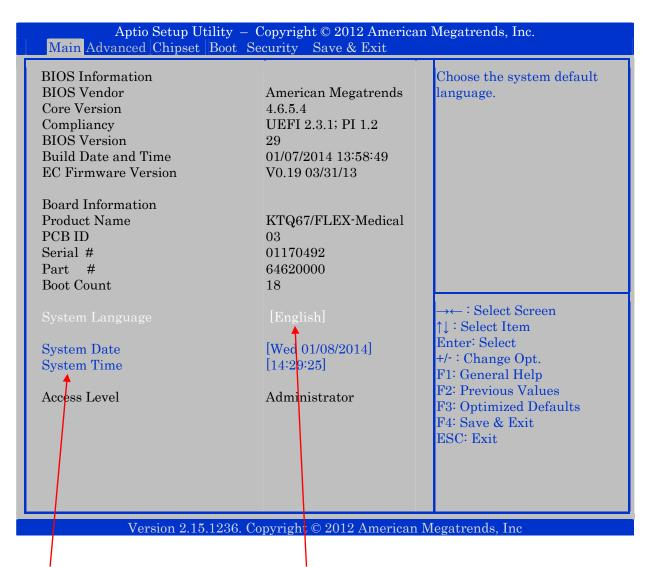
Blue text for settings that can be changed. White text for actual setting to be changed via the control keys (Black text for settings that cannot be changed via control keys)
