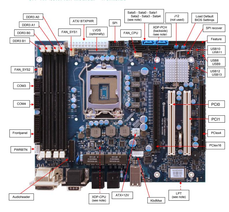
Notes: Sata0/Sata1support up to 6GB/s and Sata2/Sata3/Sata4/Sata5 support up to 3GB/S. The LPT connector and the XDP connectors are not mounted in volume production.
