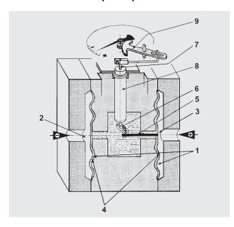
$\begin{array}{l} \text{Mounting according to affixed symbols} \\ \oplus \text{ high pressure and } \ominus \text{ low pressure} \end{array}$
