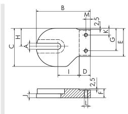
Fig.: Right bracket (A) aluminum or VA
