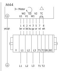
Fig.: 3-phase, winding for 2 voltages, delta connection
