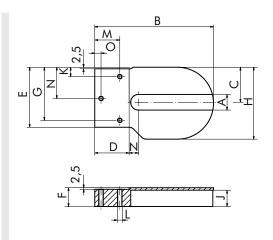
Fig.: Left bracket (B) aluminum or PE
