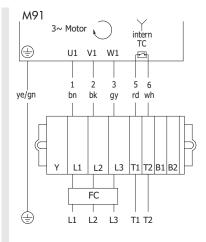
Fig.: 3-phase, 4+2-core cable, winding for 1 voltage, star connection
