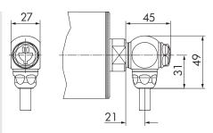
Fig.: 90° plug connection
