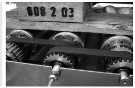
For applications without a conveyor belt or with a narrow belt covering less than 70 % of the drum motor face width, heat from the motor can no longer be dissipated via the belt contact. For these applications, we recommend using a 2-pole asynchronous drum motor or synchronous drum motor with frequency inverter.
