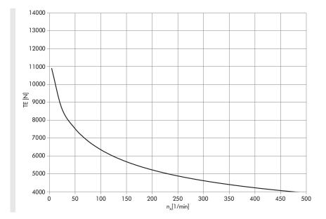
**Note:** The correct value for the maximum permissible belt tension is determined from the speed of the drum motor. When selecting the motor, also check whether the maximum permissible TE value fits the desired drum width (FW). The belt tension diagrams apply only to standard shafts.
