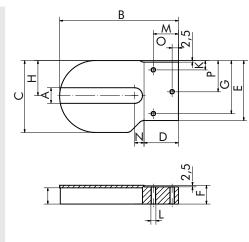
Fig.: Right bracket (C) aluminum or PE
