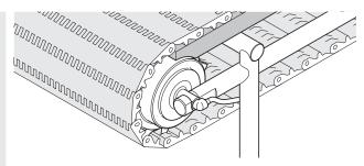
Fig.: Open conveyor design for hygienic cleaning
