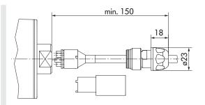
Fig.: Mounting dimensions with a mounting tool
