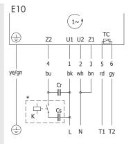
Fig.: 1-phase, 7-core cable
