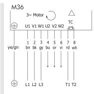
Fig.: 3-phase, 7+2 core cable, 2 speeds, delta connection
