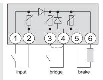
Fig.: Half-wave rectifier
