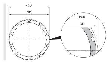
OD = Outer diameter in mm PCD = Pitch diameter in mm
