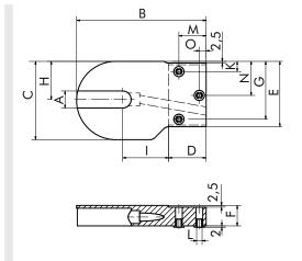
Fig.: Right bracket (A) PE for drum motor with cable connection slot
