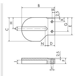
Fig.: Right bracket (C) aluminum or VA
