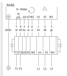
Fig.: 3-phase, 7+2 core cable, 2 speeds, delta connection
