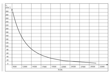
**Note:** The correct value for the maximum permissible belt tension is determined from the maximum permissible TE value for the speed of the drum motor. For motors with shell length SL > 1300 mm, check whether the maximum permissible TE value for the jacket length is lower. In this case, use the lower value as maximum permissible TE value. The belt tension diagrams apply only to standard shafts.
