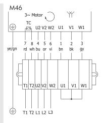
Fig.: 3-phase, 7+2 core cable, 2 speeds, double-star connection
