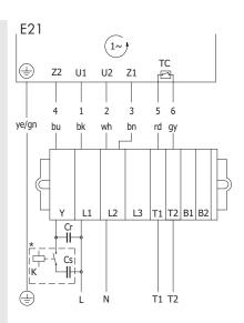
Fig.: 1-phase, 7-core cable
