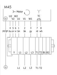
Fig.: 3-phase, winding for 2 voltages, star connection
