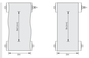
Fig.: Measuring the belt elongation
