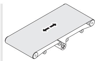
Fig.: Long belt conveyor with center drive
