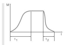
Fig.: Closing and opening response time
