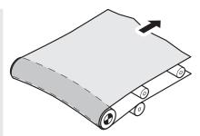
Fig.: Damaged drum motor due to over-tensioning
