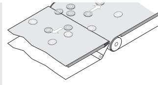
Fig.: Knife-edge conveyor
