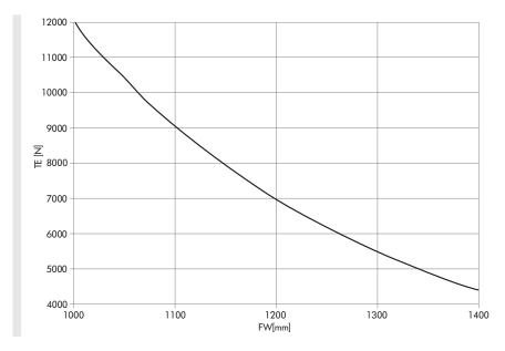
Belt tension depending on rated speed of shell
