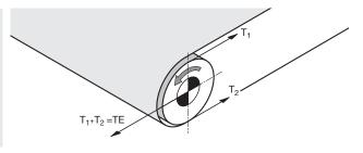
The required belt tension T1 (top side) and T2 (bottom side) can be calculated in accordance with DIN 22101 or the CEMA standard. Based on the information from the belt manufacturer, the actual belt tension can be roughly determined by a measurement of the belt elongation during tensioning.
