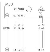
Fig.: 3-phase, 4+2 core cable, winding for 1 voltage, delta connection
