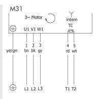
Fig.: 3-phase, 4+2-core cable, winding for 1 voltage, star connection
