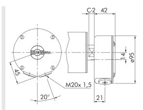
Fig.: Terminal box, stainless steel
