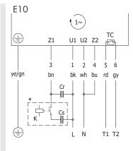
Fig.: 1-phase, 7-core cable
