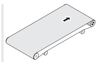
Fig.: Non-reversible conveyor with head drive
