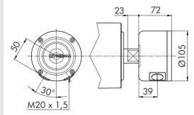
Fig.: Terminal box, techno-polymer
