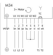
Fig.: 3-phase, 7+2-core cable, winding for 2 voltages, star connection
