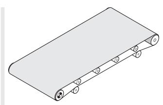
Fig.: Roller bed conveyor
