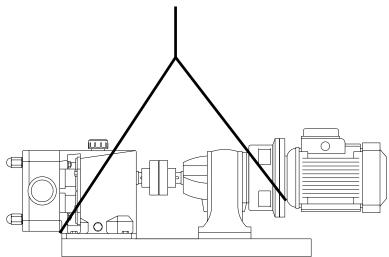
Figure 4.1: Lifting the pump.
