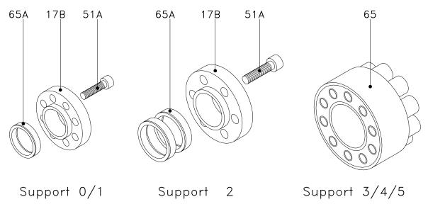
Figure 8.6: adjustable fastening mechanism
