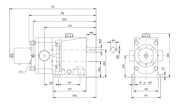
(1) Heating jacket connection 2 x R1/4" (to SLR 5) 2 x R3/8"
