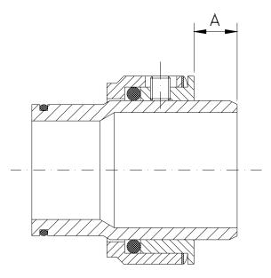
Figure 8.2: assembling the mechanical seal
