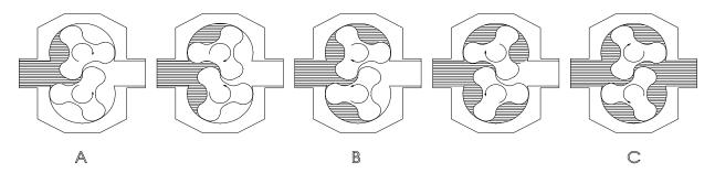
Figure 3.1: Operating principle
