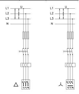
Figure 4.2: SLR pump electrical connections
