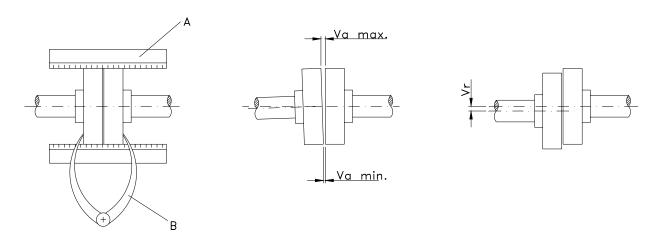
Figure 4.3: coupling alignment.
