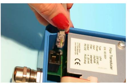
Abb. 1: PC connection with RJ22 plug with cover open
