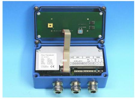
Abb. 2: LCD display connection with cover open
