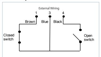
Switches shown in closed valve position. Max. cont. load 2.5 W. Insulation tested to  $1000 \, \text{V}$ .
