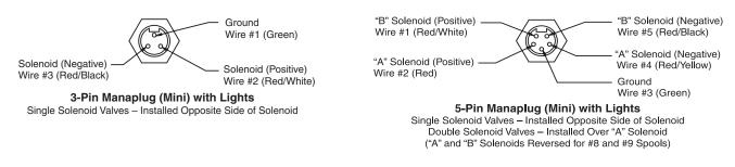
Pins are as seen on valve (male pin connectors)
