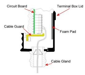
Fig 10 Cable routing
