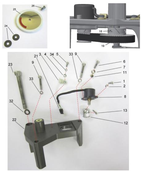
Fig 15 Sensor Mounting Bracket replacement
