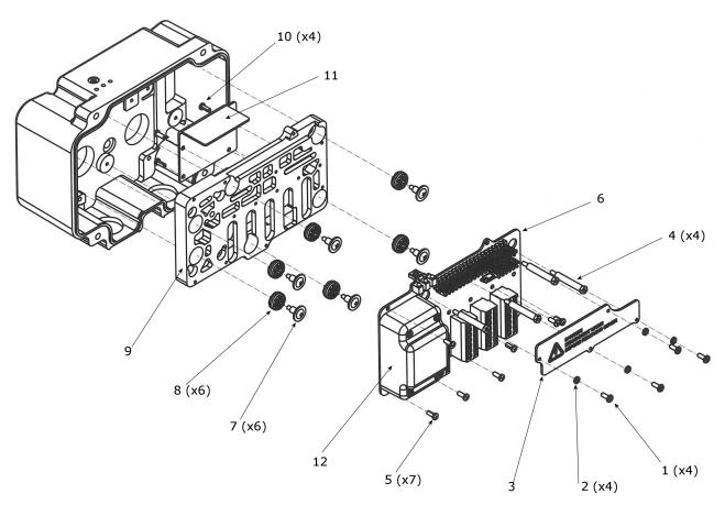
Fig 20 Terminal Board
