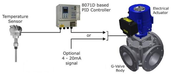
Fig 2 System Components
