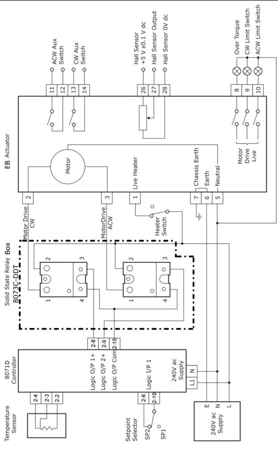
Fig 25 8071D controller with an 8073C-DDT solid state relay module
