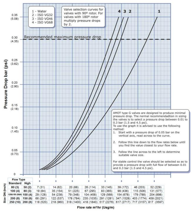
Fig 30 Valve Selection Curve
