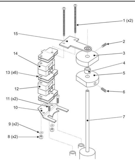
Fig 16 Limit Switch Assembly and Cams
