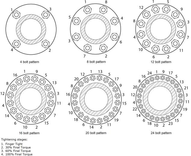
5. Final pass at 100% torque in a clockwise sequence
