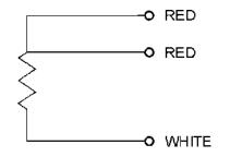
Fig 22 Temperature Sensor Connections
