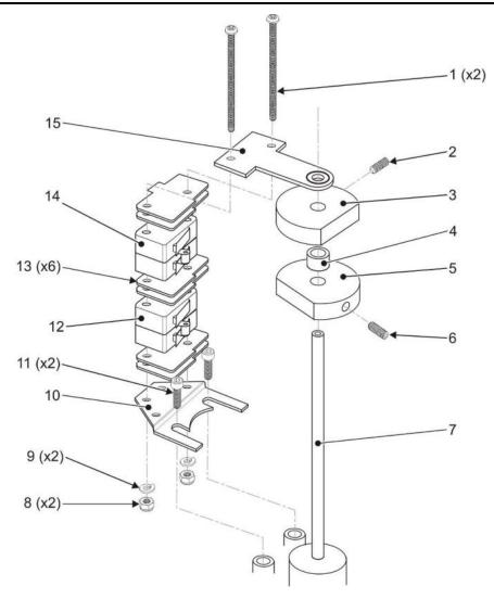
Fig 17 Limit Switch Adjustment
