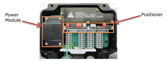
Fig 6 EB Actuator (Shown With Positioner)
