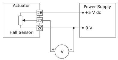
*Fig 18 Electrical Connections for Sensor Alignment*
