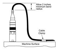
Figure 3: Cable Anchoring
