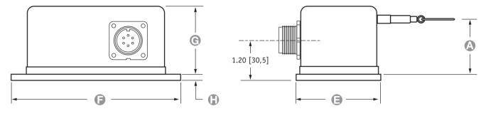
ALL DIMENSIONS ARE IN INCHES [MM]  $\cdot$  tolerances are  $\pm 0.02$  in.  $[\pm 0,5 mm]$
