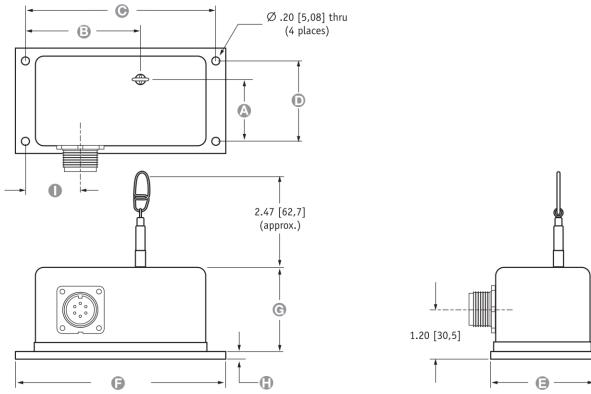
ALL DIMENSIONS ARE IN INCHES [MM] • tolerances are ±0.02 in. [±0,5mm]
