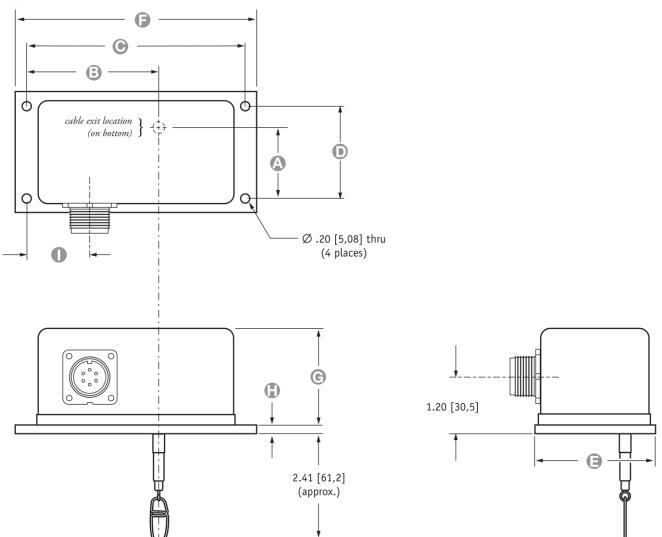
ALL DIMENSIONS ARE IN INCHES [MM] • tolerances are ±0.02 in. [±0,5mm]
