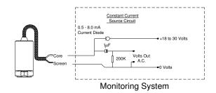
Note: Connection details for the MTN/1130QR with twin core cable vary from the above such that the core is replaced by white; screen replaced by black & the screen is then not connected.
