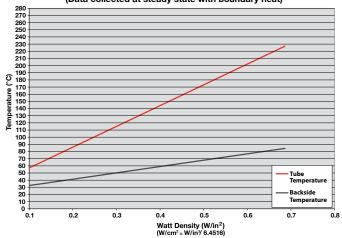
Watt Density vs. Tube Temperature vs. Jacket Backside Temperature
