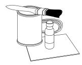
This two-part adhesive consists of a resin and catalyst that are easily mixed together and applied with a paintbrush. Recommended usage is for field cementing of silicone rubber heaters to customer parts. Available for immediate delivery, the cement kit handles temperatures up to 350°F (175°C). The resin is available in pint or quart containers. To order, specify **silicone contact cement** and the container size.
