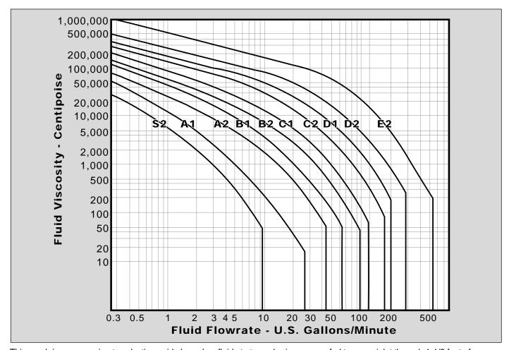
This graph is an approximate selection guide based on fluid at atmospheric pressure fed to pump inlet through 1-1/2 feet of pipe. Full details of fluid flow, viscosity characteristics, vapor pressure and pipework are required to enable accurate pump selections to be made.
