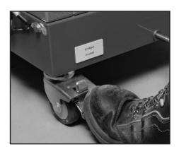
Switch off the wet separator and apply the parking brake - if fitted.
