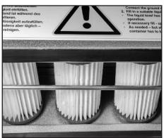
In this case, either the filters or moisture separator is dirty, or the container contains sludge.
