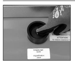
The degasification valve should always be checked for correct operation before commissioning and each time before starting the wet separator. Ensure that the machine is switched off before carrying out this check. The valve head should slot into place with gentle pressure and automatically return to its original position with the help of the spring.
