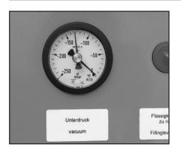
The container must be emptied and cleaned when the pointer of the vacuum gauge is above the factory set value.
