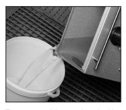
The contents of the container should be emptied out into a suitable vessel. Dispose of the vacuumed material in accordance with all applicable, national environmental regulations
