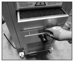
Pull the container out of the housing using the handle.
