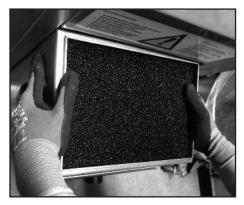
If despite being cleaned the moisture separator is still dirty it must be replaced. Remove the moisture separator from the housing. Then insert a new moisture separator.
