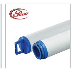
The PEACH DynaSep, Series EZ-PCHG, cartridge utilizes PEACH technology to remove deformable and shear sensitive contaminants from natural gas streams. The unique end cap design requires no tools, allowing for easy installation & removal during change-outs. The inclusion of EZ-Align® ensures a positive seal and prevents cartridge sagging. The unprecedented multi-
