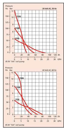
Note: Characteristics with water at 20 °C - Figures of flow are averages.
