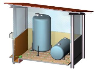
Use of a cable electrode for leakage detection in a storeroom
