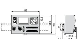
Universal controller with DIN rail TS 35 (dimensions not to scale)
