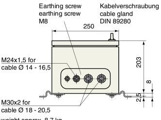
Standard control box (supply voltage 380 / 440 V - control voltage 115 / 220 V) - other voltages on request
