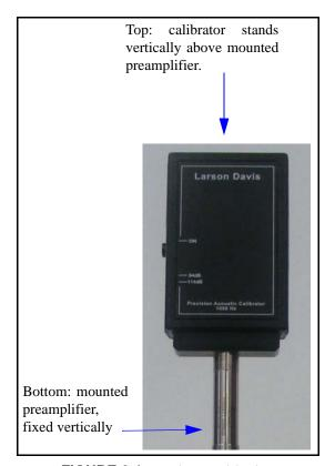
**FIGURE 2-1** Vertical Positioning
