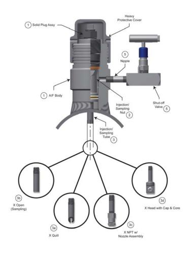
TYPICAL COSASCO® INJECTION/SAMPLING SYSTEM
