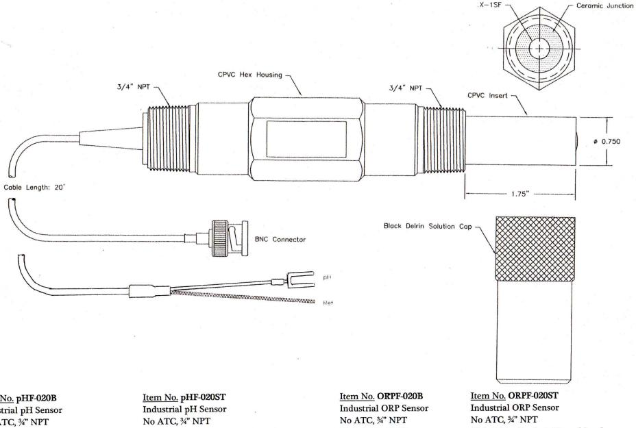
Item No. pHF-020B Industrial pH Sensor No ATC, 3/4" NPT 20-ft Cable, BNC
