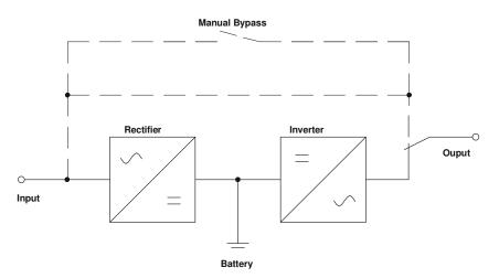
Figure 1: Block diagram "Normal operation"
