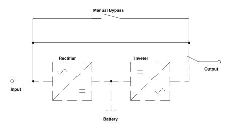
Figure 4: Block diagram "Manual bypass"
