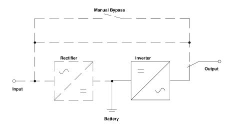
Figure 2: Block diagram "Power failure"
