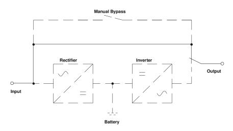
Figure 3: Block diagram "Fault in the inverter"
