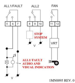
The ALL1 / FAULT relay operates normally when the unit is powered, therefore contact 5-7 is closed. The above picture shows the state of the relays in non-alarm condition.
