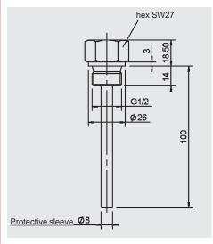
Tank mounting sleeve for ETS 3000 with integral sensor probe, probe length 100 mm Order no. 909640
