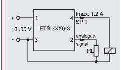
Model with 2 switching outputs and 1 analogue output:
