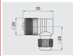
**ZBE 08-02** (5 pole) Right-angled connector, M12x1, with 2 m cable Order no.: 6006792
