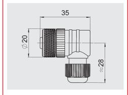
ZBE 06-02 (4 pole) Right-angled connector, M12x1, with 2 m cable Order no.: 6006790
