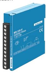
The MS220K is a particularly economical standard design in a 22,5 mm wide housing with vertically arranged terminals. Each terminal remains accessible even if all others are already occupied.
