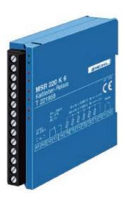
The MSR220K6 monitors up to 6 PTC-reseitor sets with up to 6 PTCs each at the same time. If a temperature rise occurs in one set, the output relay releases and LEDs show the overheated sensor.
