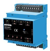
The MSF220VL is particularly suitable for monitoring of temperatures at dry transformers, when also the temperature of the core shall be measured. An intelligent control prolongs automatically the runtime of a cooling-fan, depending on the load of the transformer. Each PTC-circuit is monitored for break and short circuit. This reduces probability of false alarms. Relays in operating-current mode prevent from a trip-signal when switching on supply voltage.
