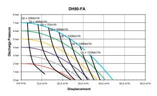
Curves are based on internal Air Valve only
