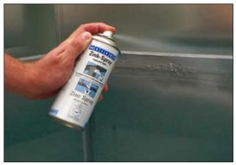
WEICON Zinc Sprays are dust-dry after about 15 minutes and can be spackled and painted over after about 12 hours without pretreatment. The temperature resistance amounts to up to +500°C (in the case of "bright grade", up to +300°C).
