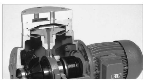
Cutaway - Double diaphragm pump
