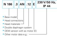
In addition the motor data must be given in the purchase order (voltage, frequency, and protection class). In our extensive program you are sure to find the pump you need for your particular application.
