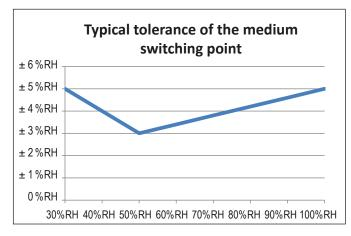
1-point-adjustment at 48 % RH/23 °C Long-term drift: ≤±1 % RH p.a.
