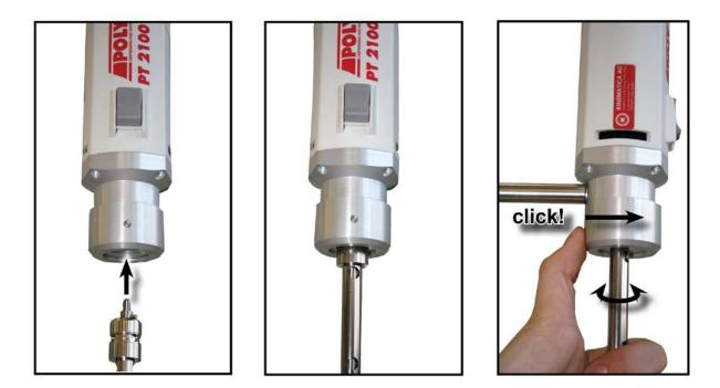
The connection of aggregates is effected without tools by a safety quick-coupling. The aggregate has to be inserted into the motor-side coupling and slightly turn into ist correct position only – until you hear a clear "click".
