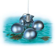
If, for example, oil flows onto a still water surface following a leak, exact setting of the rod electrode will ensure that an oil layer of only approx. 3 to 10 mm thickness is sufficient to interrupt the control current flowing via the rod electrode and activate an alarm.
