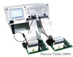
The Tracker 2800S can scan and compare up to 40 pins per channel using standard IC clips and cables. Connections are made through the front panel using standard IDC style connectors. Comparison can take place manually or automatically
