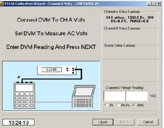
Channel A mid range AC calibration Next, click in the Voltage Reading window and enter the reading of the voltmeter. Verify that the correct units (Pk, Pk-Pk, or RMS) are selected for the type of voltmeter you are using.
