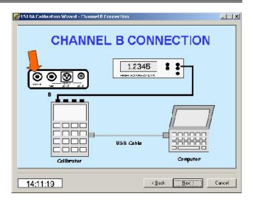
Channel B Low range AC calibration Next, click in the Voltage Reading window and enter the reading of the voltmeter. Verify that the correct units (Pk, Pk-Pk, or RMS) are selected for the type of voltmeter you are using.
