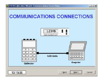
The next step in the Calibration Wizard uploads the units' serial number and software version information. Verify these numbers with those found on the label affixed to the back of the unit.
