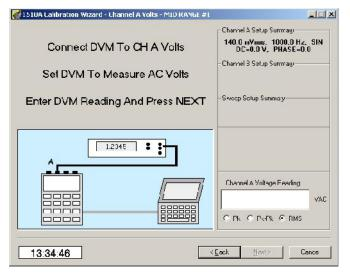
Channel A high range AC calibration Next, click in the Voltage Reading window and enter the reading of the voltmeter. Verify that the correct units (Pk, Pk-Pk, or RMS) are selected for the type of voltmeter you are using.
