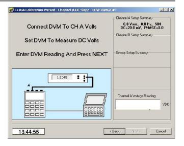
Channel A mid range DC calibration Next, click in the Voltage Reading window and enter the reading of the voltmeter. Verify that the correct units (Pk, Pk-Pk, or RMS) are selected for the type of voltmeter you are using.
