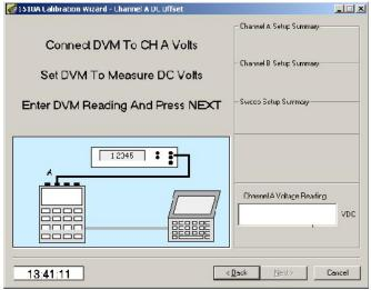
Channel A DC low range calibration Next, click in the Voltage Reading window and enter the reading of the voltmeter.
