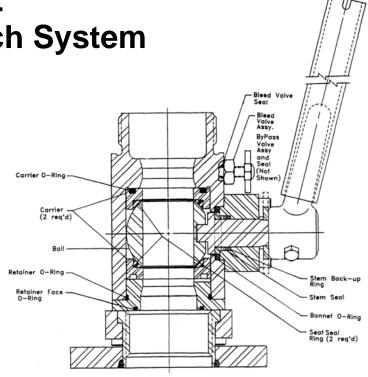
Service Valve configuration is shown in Figure 1. The retriever end connection is a three and one-half inch acme thread, mating with the hammer nut of the RBS/RBSA/RSL Retrievers. At the other end, a three inch acme thread hammer nut mates with the COSASCO<sup>®</sup> Access Fitting.
