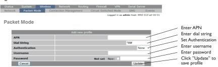
Note: In order to set a password click the check-box marked New. The password can now be entered in the text field. The password is visible as it is being typed so that it can be checked for errors prior to being set. Once set the password will no longer be visible.
