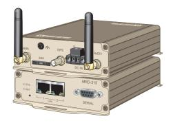
using the built-in two port Ethernet switch and the RS-232 D-sub.
