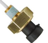
The **Model S85** is an active device which is designed to give an alarm signal if liquid falls below / rises above a preset level. It will only signal an alarm after a few seconds of low / high level to eliminate false alarms due to turbulence.
