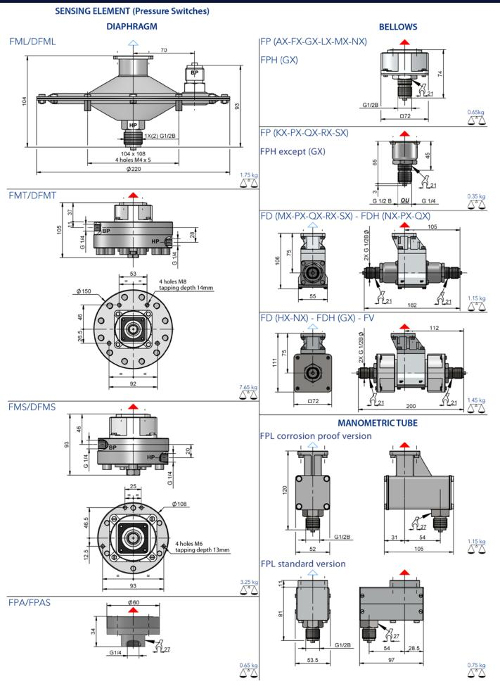
The weights given are approximate and as a rough guide only and may vary according to the designs. The weight of the FC type thermostatic element is indicated for a 2-metre capillary. Dimensions are given in mm.
