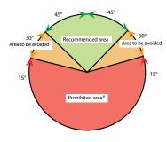
Recommended area: ±45° either side of the vertical axis, bulb down (capillary output up).
