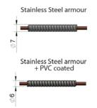
For all ranges greater than 125°C the sheath length is 10 to 20 cm less than that of the capillary.
