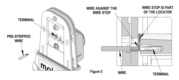
Note: The tamper proof ratchet action will not release the tool until it has been fully closed.
