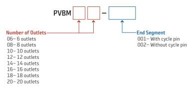
The PVB Divider Valve features a smart part number ordering system. Choose the number of outlets and the type of end segment. For example: To order a 6 outlet divider valve with a cycle pin, you would use Part #PVBM06-001.
