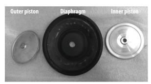
Pic. 6: Diaphragm with piston fixture
