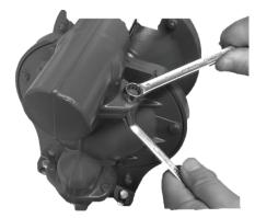
Pic. 1: Disassembling of the manifolds
