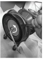
Pic. 4: Diaphragm disassembly
