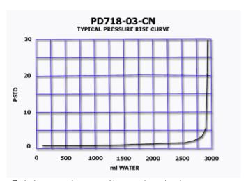
Typical pressure rise curve with water absorption demonstrates the nearly flat low pressure drop curve until the cartridge is nearly saturated.
