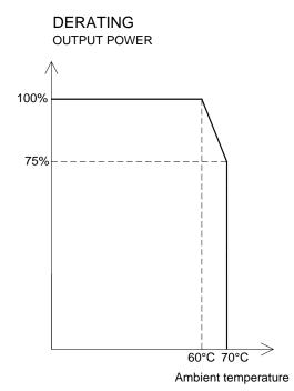
To prevent overheating of the unit, the consumer load must be reduced equivalently.
