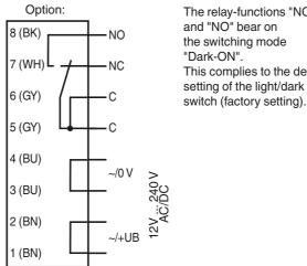
The relay-functions "NC" and "NO" bear on the switching mode "Dark-ON". This complies to the default setting of the light/dark
