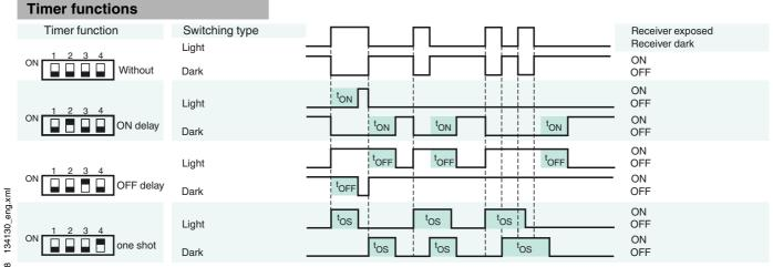
Time  $t_{ON}$ ,  $t_{OFF}$  and  $t_{OS}$  are adjustable from 0.1 to 10 seconds. The Light-/Dark-Switch (Left, outer switch) is shown in the "Dark ON" position.
